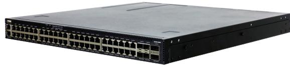
The Edgecore EPS203 is a high-performance Gigabit Ethernet Layer 3 switch featuring 54 ports. The EPS203 has 36 x 10/100/1000/2.5G ports, 12 x 10GBASE-T ports, 4 x 25G uplink ports and 2 x 100G QSFP28 stacking ports (stacking capability subject to NOS implementation); plus all RJ-45 Ethernet ports can support up to 90 W Power-over-Ethernet (PoE).
